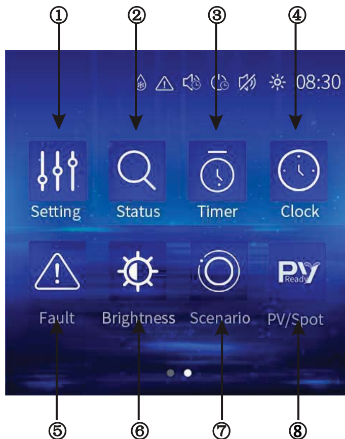
Figure 16: Control Panel Menu Screen
