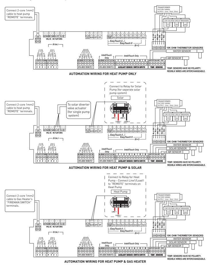
Figure 16: Automation Connections
