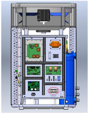
Figure 12: Inside View of Electrical Box.
