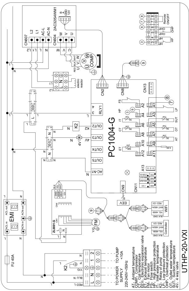
Figure 18: Wiring Diagram - UltraTemp 20kW VXi models
