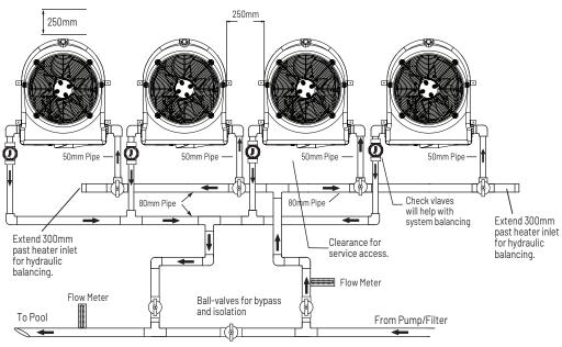
Figure 9: Multiple Heat Pumps Configuration Page 14
