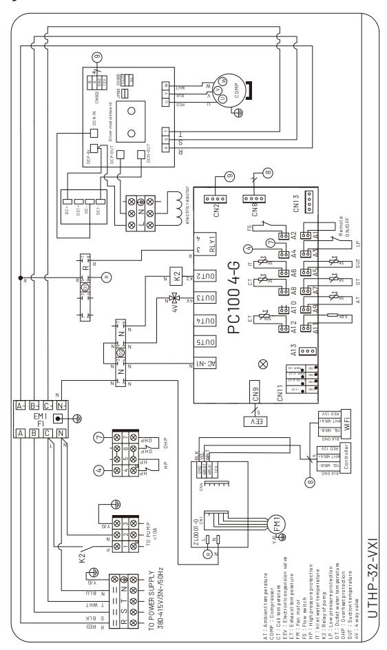
Figure 21: Wiring Diagram - UltraTemp 32kW VXi models
