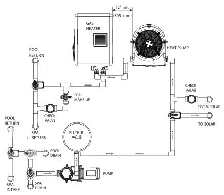
Figure 8: Multiple Heat Source Configuration
