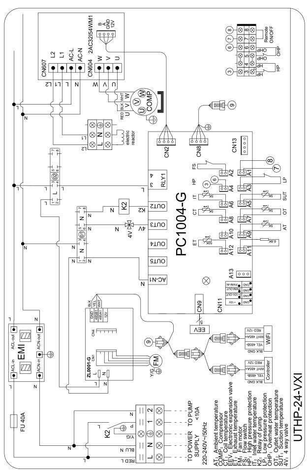
Figure 19: Wiring Diagram - UltraTemp 24kW VXi models
