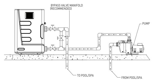
Figure 6: Plumbing Connections - Separate Circulation System
