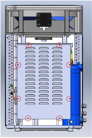
Figure 11: Electrical Cover Panel. Remove.
