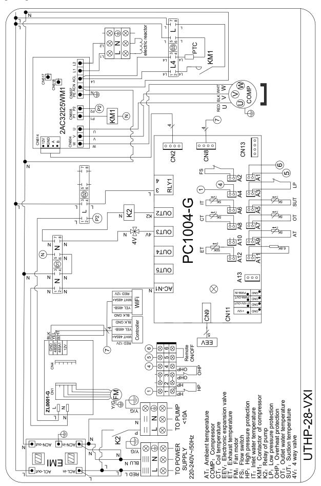
Figure 20: Wiring Diagram - UltraTemp 28kW VXi models
