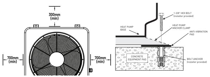
Figure 3: Anchor Clamp Installation
