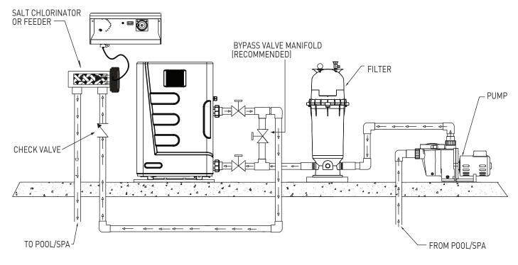
Figure 5: Plumbing Connections - Standard Circulation System
