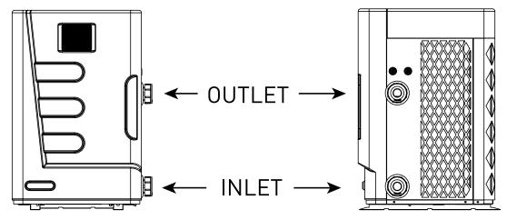
Figure 4: Water Connections to the Heat Pump
