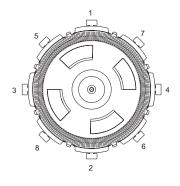
FIGURE 5 - 25" Filter clamp tightening sequence.
