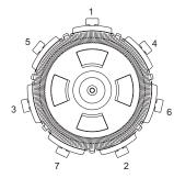
FIGURE 4 - 21" Filter clamp tightening sequence.
