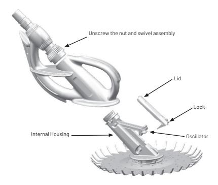
To remove damaged or worn Oscillator; no tools are required. Simply grab the Oscillator, pull and waggle outward until it unclips from the steel pin. To install the new Oscillator push it in firmly (TOP side up as marked) onto the steel pin until it snaps in place. If the Oscillator is clipped in the wrong way (TOP side down) you will not be able to close the lid.
