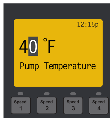
Setting the Anti Freeze Pump Temperature
